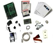
Use this economical system to perform traditional debugging activities such as executing code in run or step mode, setting break points, monitoring or modifying CPU registers, memory and application variables, and creating log or script files to record test results or create test suites. CodeWarrior supports MMEVS.
