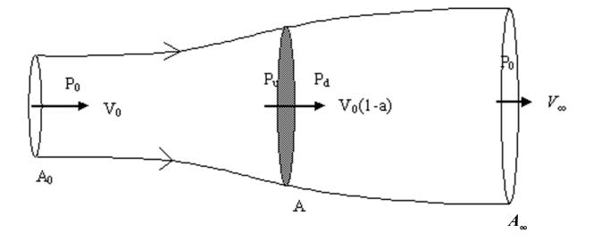
Assuming that the air is incompressible, and that it behaves as an ideal fluid except where it interacts with the windmill, use Bernoulli's equation to find the pressure discontinuity  $\Delta P = P_u P_d$  as a function of  $\rho$ ,  $v_0$ , and .
