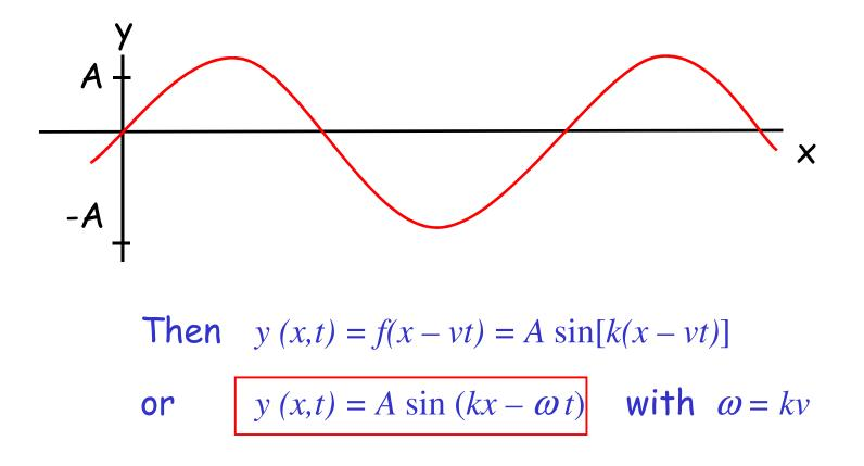
The displacement of a particle at a fixed location x is a sinusoidal function of time - i.e., simple harmonic motion:
