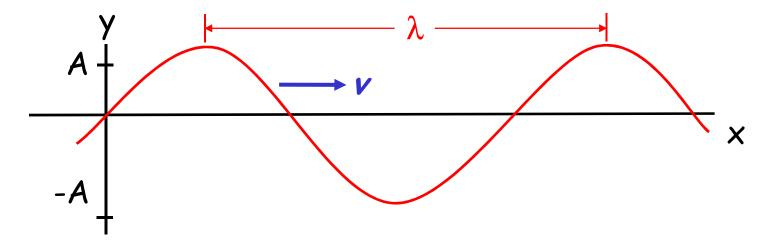
$\lambda$  ("lambda") is the wavelength (length of one complete wave); and so (kx) must increase by  $2\pi$  radians (one complete cycle) when x increases by  $\lambda$ . So  $k\lambda = 2\pi$ , or
