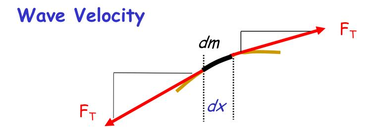
Exercise: show that the net vertical force on the short element of rope (of length dx) is, approximately, given by
