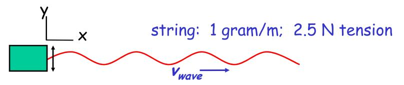
Oscillator: 50 Hz, amplitude 5 mm
