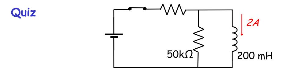
There is a 2A current through the inductor, and the switch is suddenly opened. What is the voltage across the inductor immediately after the switch is opened?
