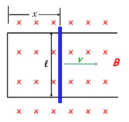
We can derive the same expression,  $\mathcal{E} = B \ell v$ , from Faraday's Law, if we keep track of a complete circuit. Consider a conducting bar sliding along a a U-shaped conductor as shown.
