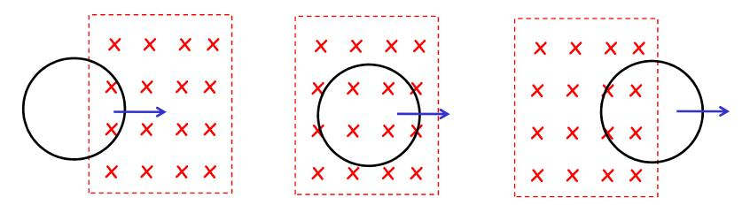
The circular wire moves at constant speed through the region of magnetic field. The induced emf in the wire during this time
