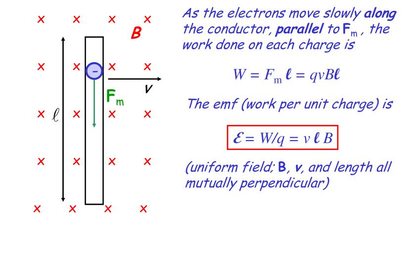
As the electrons move slowly along the conductor, **parallel** to  $\mathbf{F}_{m}$ , the
