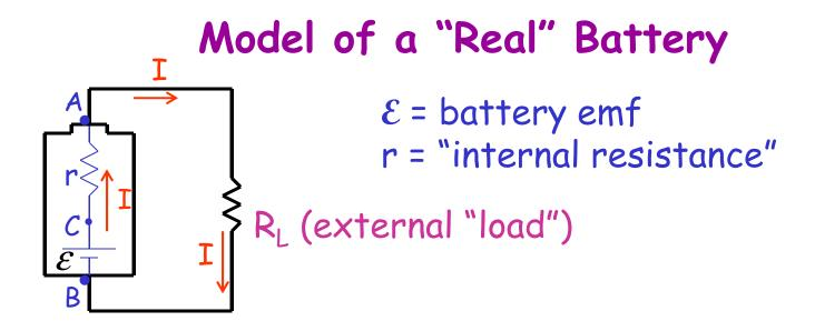
$V_A - V_B =$  "terminal voltage"  $\rightarrow$  measured
