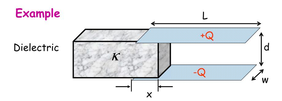
A dielectric is slid into the space between the plates of a charged capacitor.
